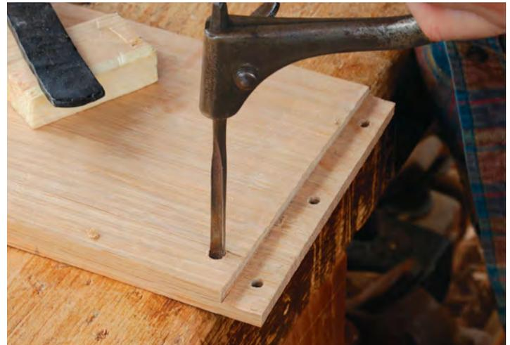
**Holes for pins and pintles.** The rabbets get pinned, so bore those holes in the box front and back now. Also bore the clearance hole for the pintles on the till's lid. This hole should not sit too close to the box's upper edge or the rabbet.
