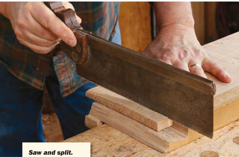
**Saw and split.** After sawing the rabbets' shoulders, Follansbee splits the cheeks. The grain must be straight for this to work well. Stay well shy of your depth layout line.
