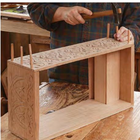
**Add the till parts and front.** Drop the till parts dry into the back, with the till lid open. Apply glue to the box ends and put the front in place. Patiently fiddle the till parts into position in the front, then drive the pins.
