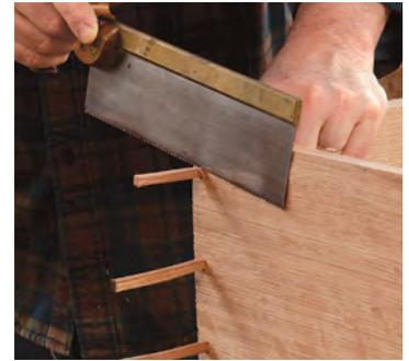
**Square pins, round holes.** Pin the back first. Use straight, square pins slightly larger than your pilot holes. The ideal pin compresses the hole a bit and fills it completely. Trim and pare the pins flush afterward.
