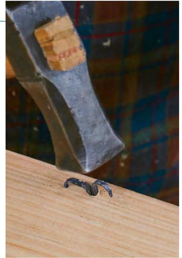
**Install the hinge in the lid.** It's easiest to press the lid onto the hinge from above. A piece of scrap protects the lid from the hammer blows. When that's done, clinch the hinges in place.
