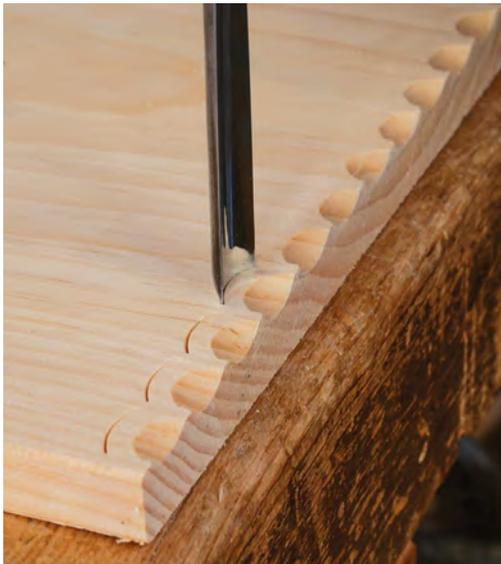
able to fit the bottom board to the box you made, not the one you planned. Place the box carcass on top of the oversize bottom board with the two flush at the back. Scribe around the box sides, inside and out. Then mark the overhang.
