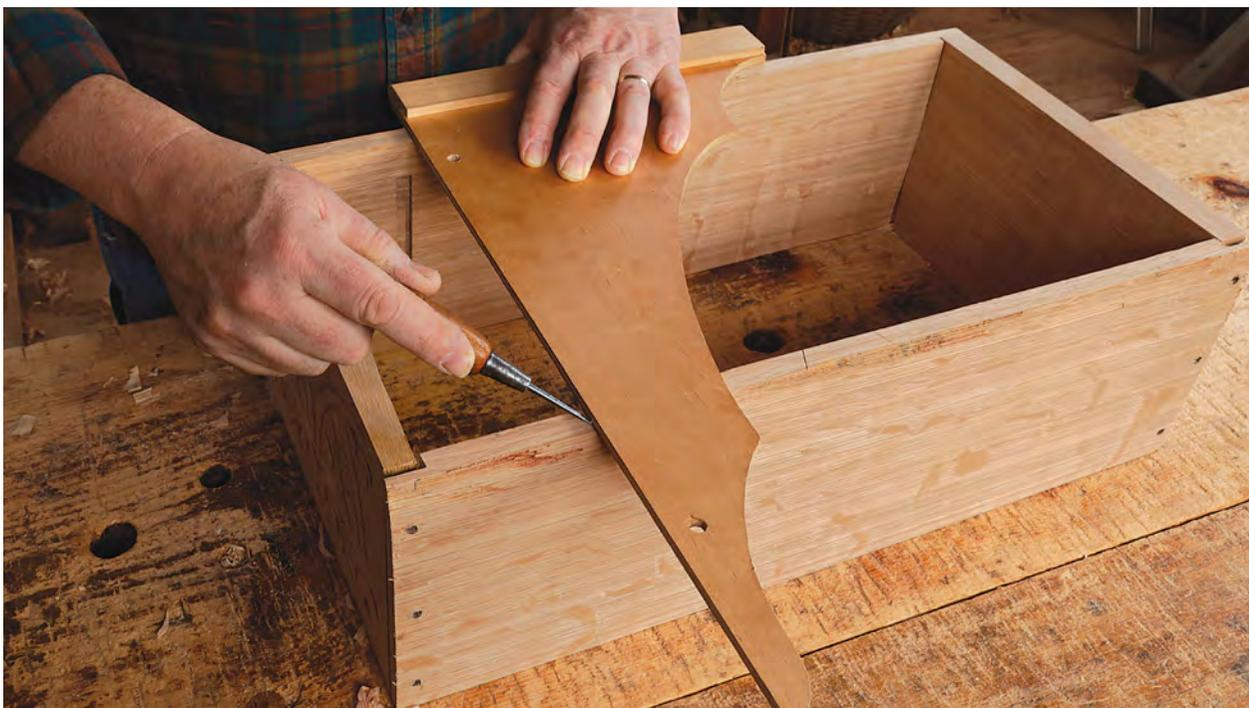
**Mark till lid's length and pintles.** Having the box clamped up to do this lets you mark off the actual piece instead of relying on a drawing.
