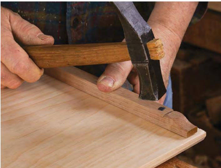
**Nail cleats to the top.** Because Follansbee uses a wide single board for the lid, he uses cleats to help keep it flat. These have decorative ogees at the front. Drive overlong nails through the cleat and the top.
