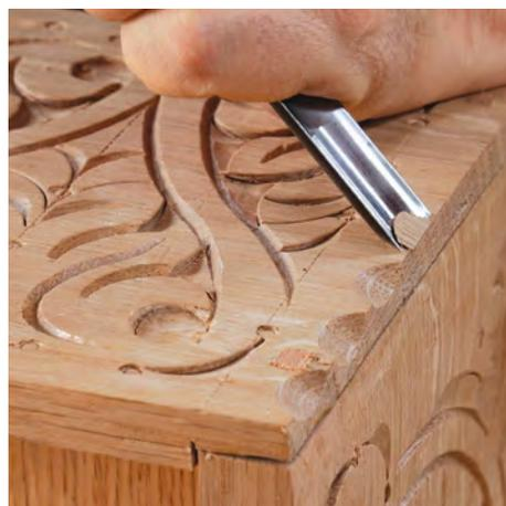
**Carve the thumbnails.** Use a deeply curved gouge and a mallet to chop thumbnail cuts into each end of the box front. Then use the same gouge to punch an echo cut right behind each thumbnail. Eyeball the spacing.
