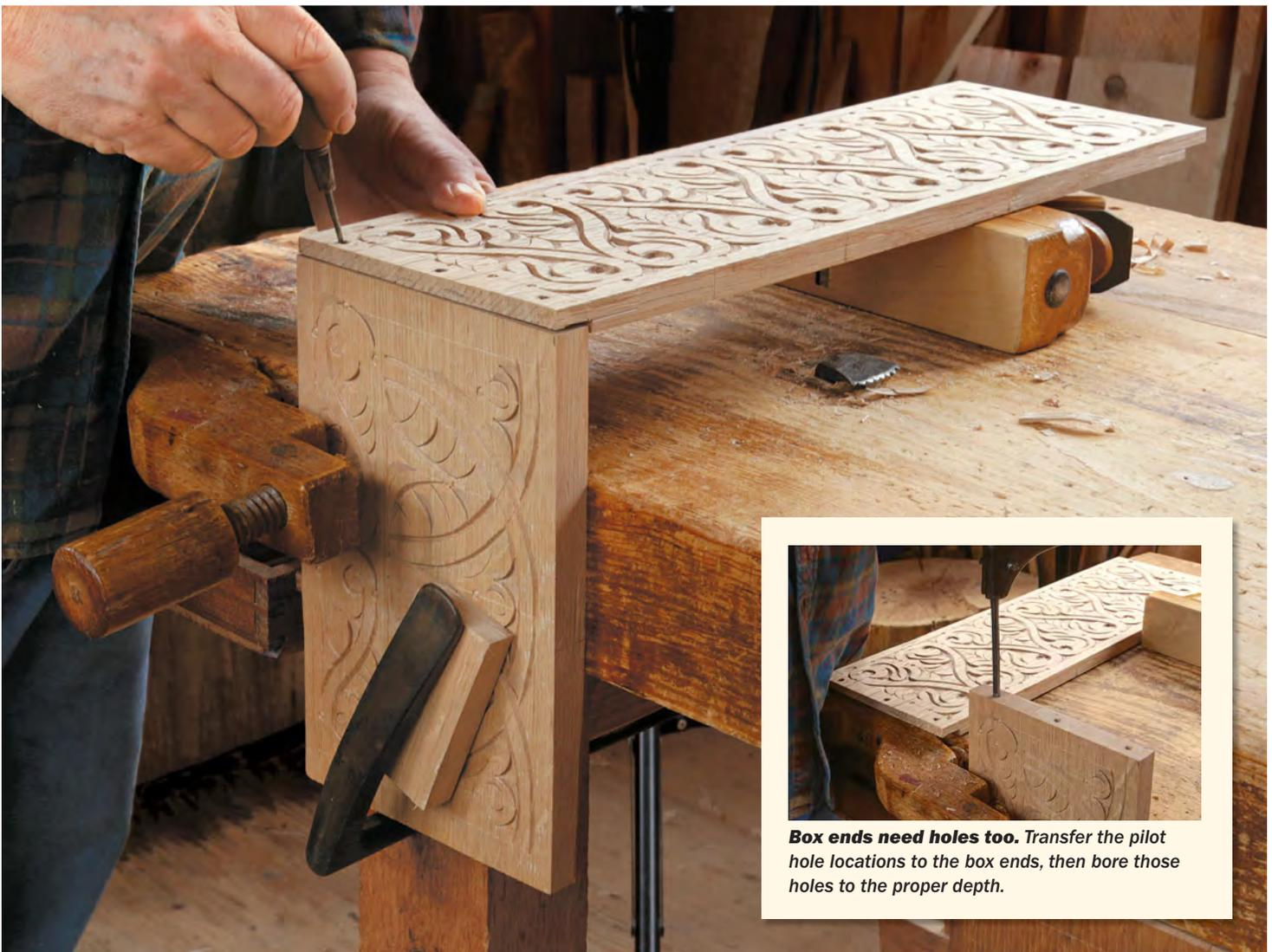
**Box ends need holes too.** Transfer the pilot hole locations to the box ends, then bore those holes to the proper depth.
