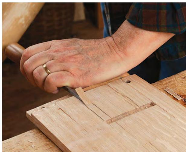
**Transfer the till joinery with the box assembled.** To lay out the till joints on the back of the box, first extend the dado's layout to the top edge of the front. Then use a large square to scribe those marks on the back side. Lay out the groove with a marking gauge. Then cut the till joints.
