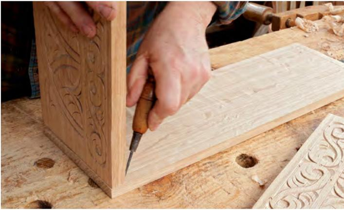
**Mark each rabbet with its matching box side.** If you prep these boards by hand, you likely won't get both ends exactly the same thickness. So mark each rabbet using the part that will join it.
