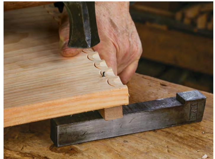
**Clinch the nails with a hard backstop.** After bending the nail's tip over, hammer it back into the lid. Use a metal stop, like this benchdog, to back up the nail head.
