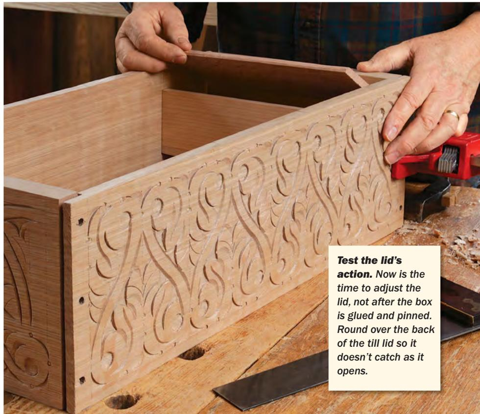
**Test the lid's action.** Now is the time to adjust the lid, not after the box is glued and pinned. Round over the back of the till lid so it doesn't catch as it opens.
