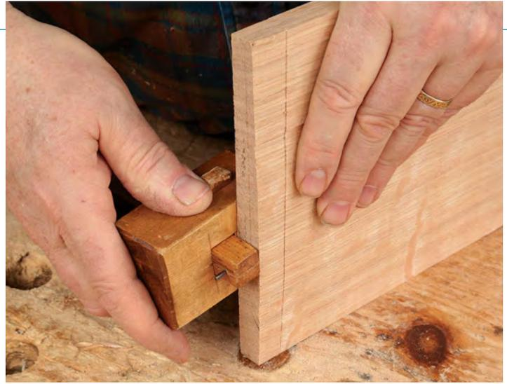
**Marking gauge lays out rabbets' depth.** Reference off the same surface for each joint. Follansbee uses the outside faces.
