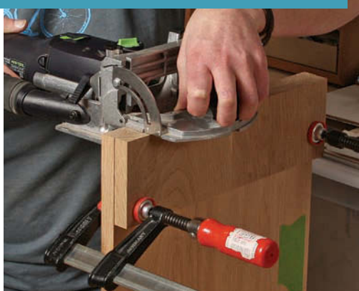
REMOVE SHIM AND MORTISE THE SIDE
