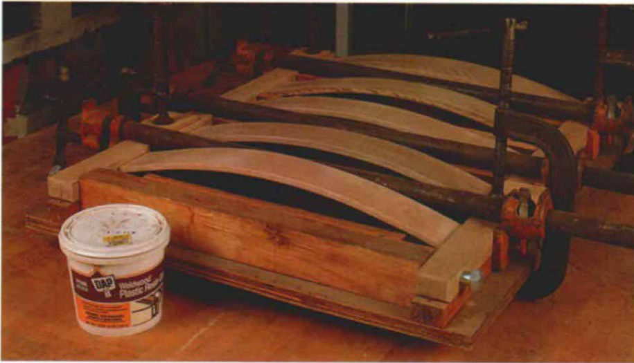
Back parts fit into a clamping fixture to keep everything straight during glue-up. Bolts through the back postpeg holes not only help align the parts in this fixture, but they are used to index the back posts in another fixture for cutting the slat mortises.
