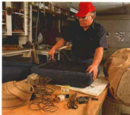
Stapling the bottom of a seat cushion , the author finishes the upholstery work for his Morris chair. Upholstery materials such as the cotton batting (right) or webbing and springs (foreground) are available from local upholstery supply stores.
