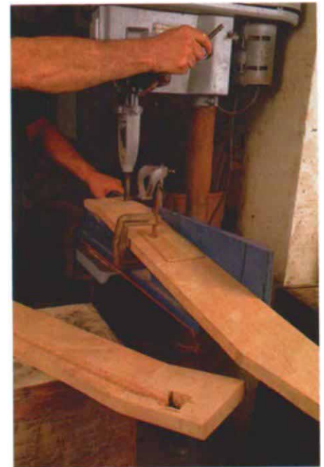
Using a hollow-chisel mortiser attachment on the drill press makes quick work of cutting the through-mortises in the chair's arms to take the leg tenons. The same device also works to cut the groove under the arm to fit on the side rails, as shown on the already-cut arm in the foreground.
