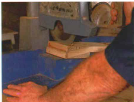
A radial-arm saw cuts away waste (below) to form the bend in a chair arm after a block of wood was glued underneath. An angle block holds everything in position.
